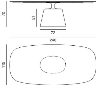
The height of H72 has a dimensional tolerance of  $\pm$  cm. Variations are to be considered, especially for tables with cement tops.
